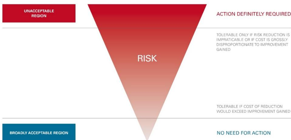
Figure 2: Illustrating the ALARP concept (after ISO 31010)
