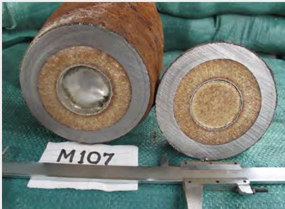
Cutting shows that the rust on the surface of projectile #8 is superficial and that the casing is in good condition
