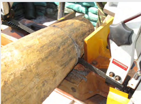
Cutting the nose section, complete with fuze, of an Mk 82 bomb. While most Mk 80 series bombs found in Vietnam will have a superficial layer of rust, the thick steel casing is unlikely to be penetrated for many years to come
