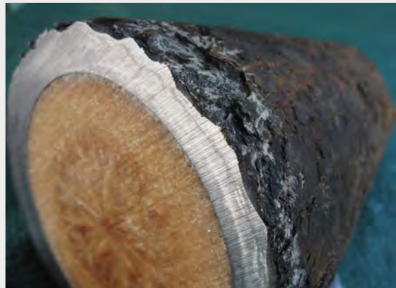
The surface of projectile #7 is heavily pitted. Nevertheless, a substantial proportion of the casing thickness remains
