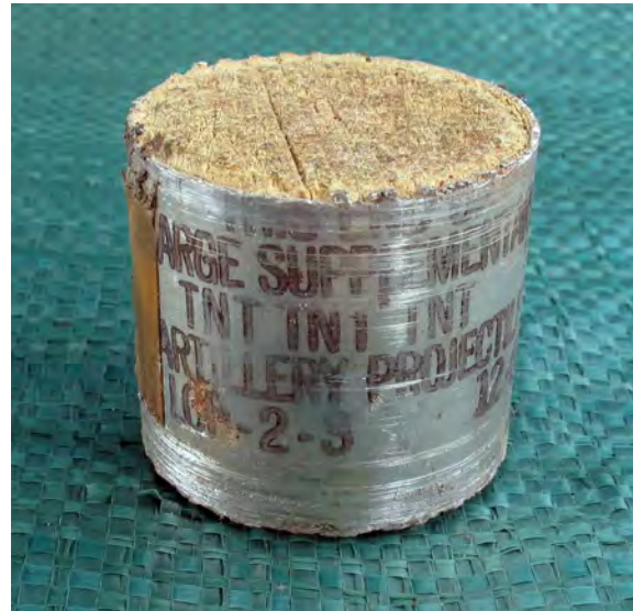
A pressed booster from a US artillery projectile, still in exceptionally good condition
