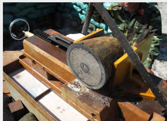
As expected, the explosive filling of the Mk 82 and Mk 84 bombs remained in good condition, protected by the thick steel casing. The explosive is likely to remain viable as long as the casing remains intact
