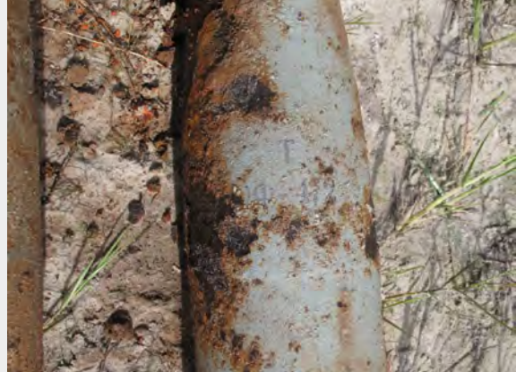
Markings, showing the designation and filling, are still just visible on the projectile surface that was lying uppermost. These would soon be lost with continued ageing
