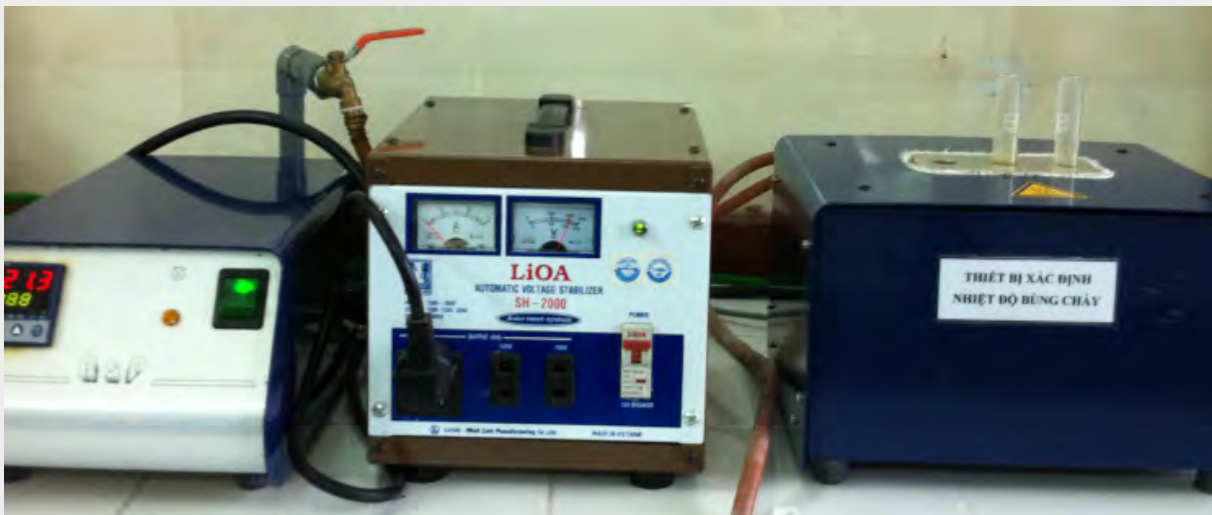
Figure 2. Flammable (burning) temperature determination device DT-400 (Germany).
