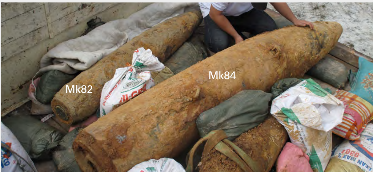
The Mk 84 bomb, along with two Mk 82 bombs, being delivered to the site. All of the bombs were fitted with an M904 nose fuze and no tail fuze. Tail assemblies were missing, as is often the case; these tend to become detached as the bomb enters the ground
