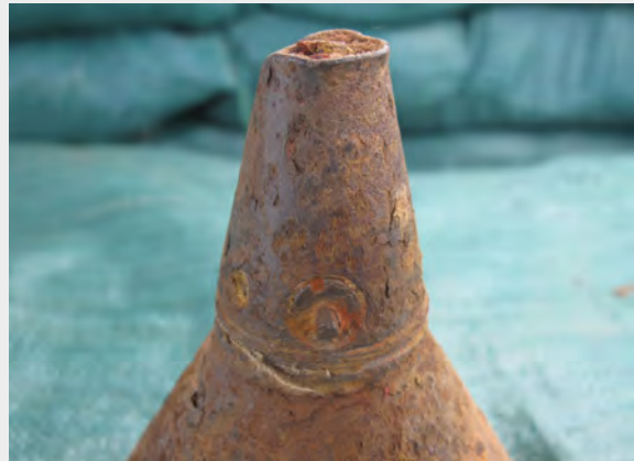
Most of the fuze was present, but damage would almost certainly have permitted water to enter. The fuze was not cut, so no internal analysis could be made
