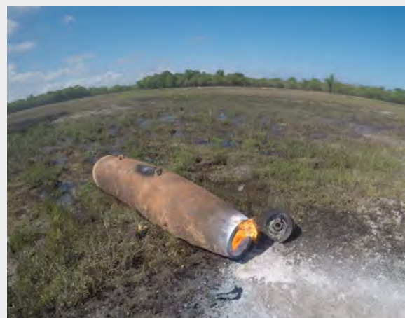
After the cut, the Mk 84 2,000 lb bomb was burned out along with the nose section containing the fuze; the Mk 84 bomb contains 429 kg of either Tritonal or H6 filler (this particular bomb contained Tritonal) and it took 40 minutes to burn out; the nose fuze detonated as required during the burnout. The image on the right shows the intense heat on the inside of the bomb casing even after the burn; note the bomb section that was cut off, containing the M904 nose fuze which was destroyed during the burnout process, to the right of the body.
