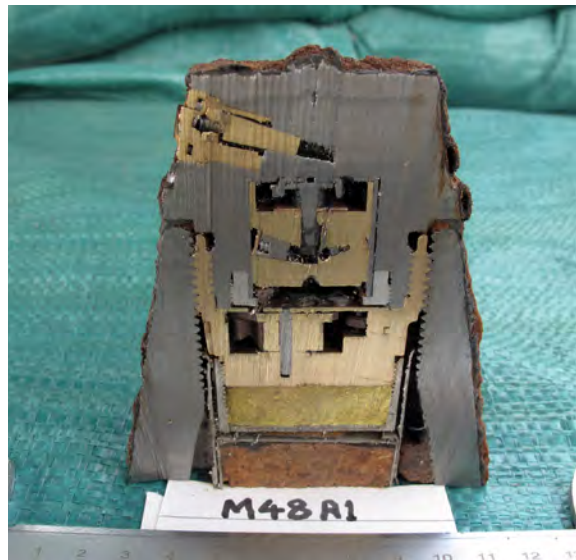
A sectioned M48A1 fuze from an M107 projectile
