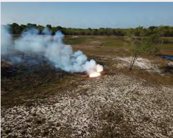
Burning out the main bodies of the 2 x Mk 82 500 lb bombs; the burnout lasted 22 minutes
