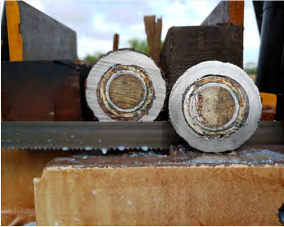
Views of the cut of the US M525 PD fuze and the booster cup section of the M374 81 mm mortar; note the damage and expansion due to corrosion of the aluminum of the fuze
