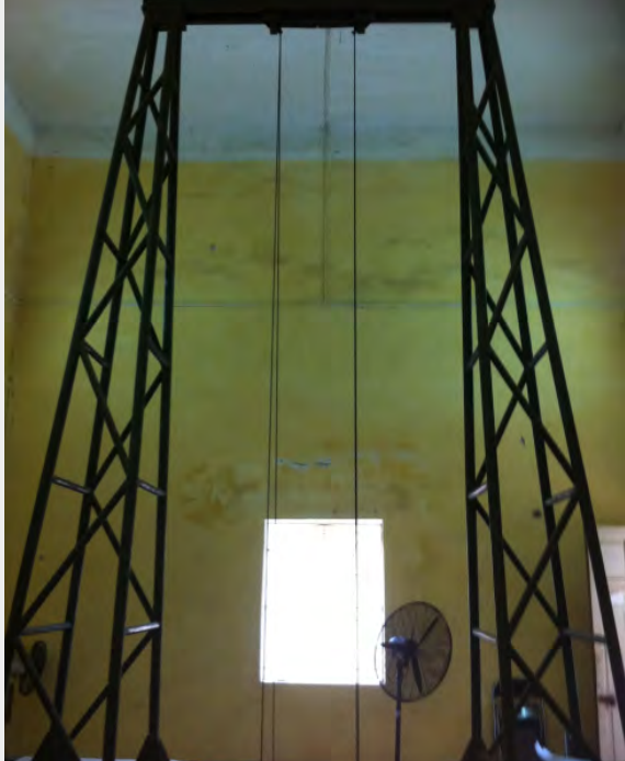
Figure 5. Determination of the ability to explosion energy with the articulation pendulum.
