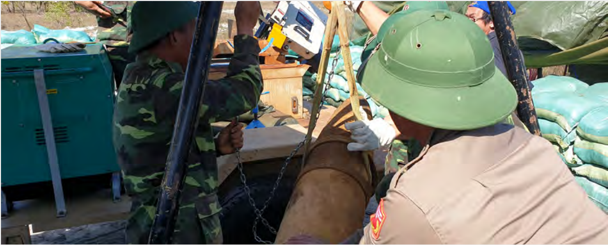
Hoisting the Mk 82 500 lb bomb onto the MCS, a single 1-ton hoist with chain was used
