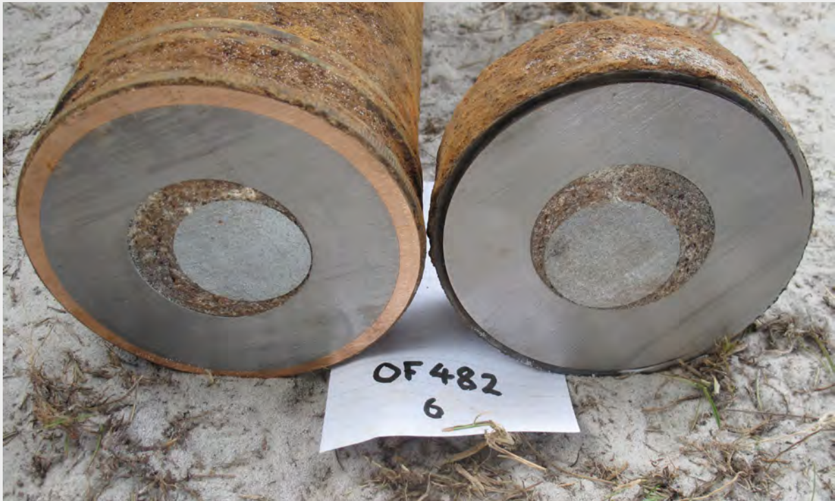
A section through the base of a 130 mm OF 482 projectile showing (left, from the outside moving inwards) the copper driving band, the thick steel casing of the base section and the lower extremity of the main charge, with embedded aluminium-based incendiary pellet
