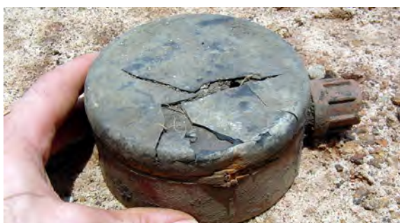
The hardening of rubber and rusting of steel have changed the characteristics of this PMN mine
