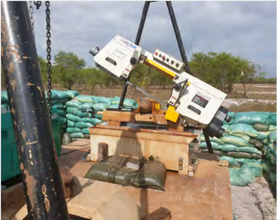
Cutting of the USSR F-853U 160 mm mortar with the GVMZ-7 PD fuze
