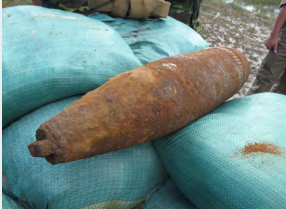
What appears to be a plug in the nose of projectile #8 is actually the remains of an M48A1 fuze
