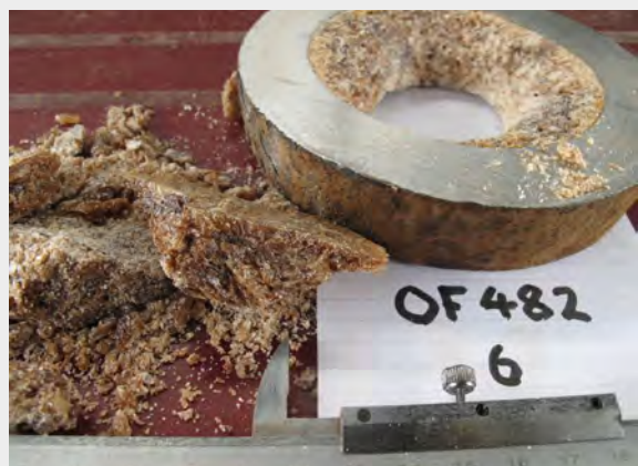
The crushed and discoloured filling of projectile #6; it is not known whether this would affect its performance
