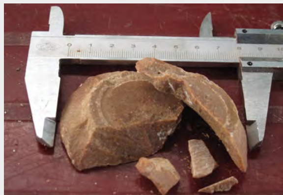
Despite cracks and cosmetic changes to the explosive, the Composition B (RDX/TNT) filling in all M374 mortar bombs was otherwise unchanged. While stable, it is capable of detonation if subjected to extreme heat, shock or friction
