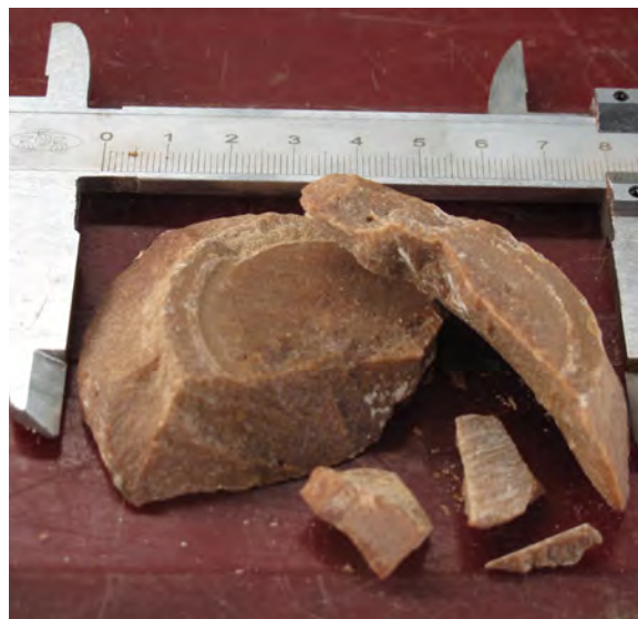
Explosives such as Composition B remain stable for long periods, but may crack on impact
