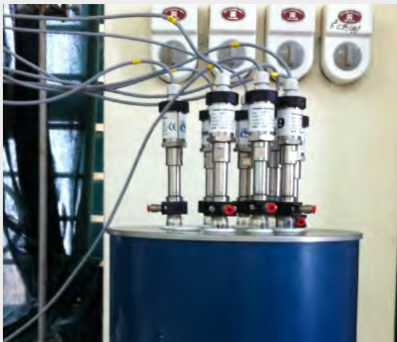
Figure 3. Vacuum stability tester (Czech) determines chemical stability under vacuum thermal stabilization method:
