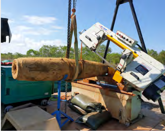
Hoisting and setting in place the Mk 82 500 lb bomb for cutting; note the use of the bomb cradle to help support the bomb as well as keeping the hoist cables connected while cutting. Each of the Mk 82 500 lb bombs had a crushed M904 PD fuze and there was no tail fuze in either one. We cut between 20 cm and 25 cm so that the booster cup was not cut through and still allowed us to make the cut large enough for the burnout process
