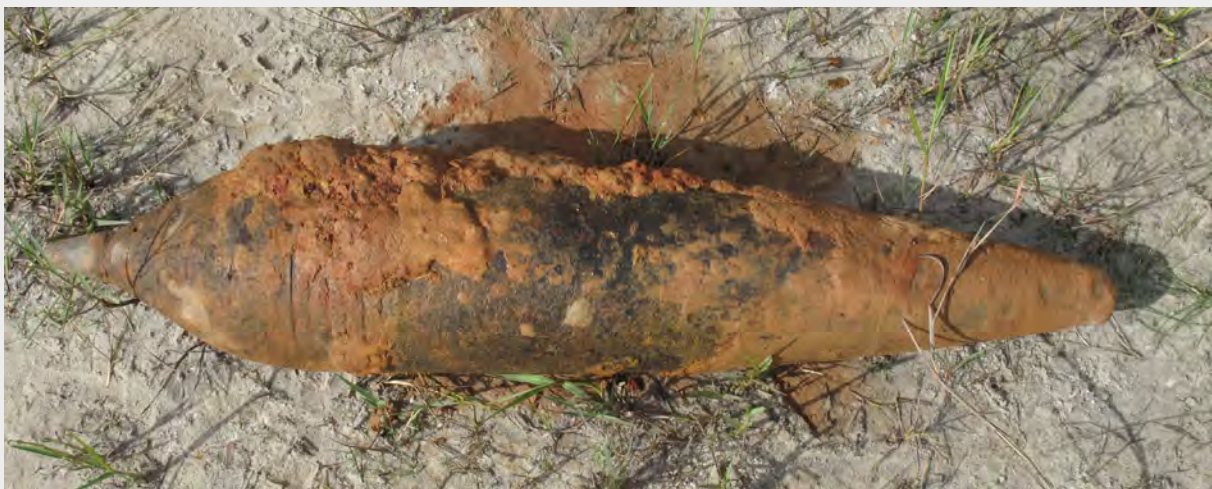
The F-853U mortar bomb presented for cutting. The body shape is distinctive enough to allow for identification despite the absence of the tail assembly; however, the missing tail makes it harder to establish whether the mortar bomb was unfired or unexploded
