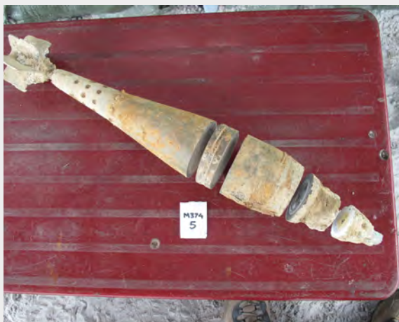
Cuts through one of the M374 mortar bombs
