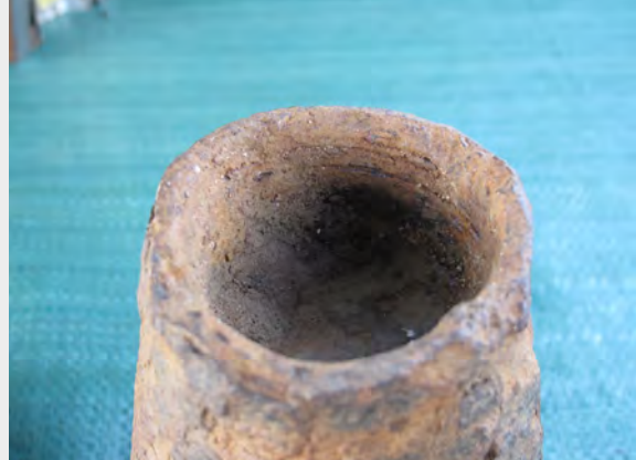
The impact of projectile #7 has removed most of the fuze body
