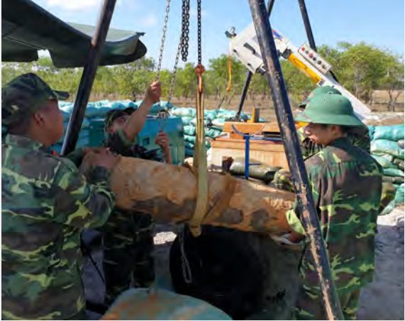
Hoisting and setting in place the Mk 82 500 lb bomb for cutting; note the use of the bomb cradle to help support the bomb as well as keeping the hoist cables connected while cutting. Each of the Mk 82 500 lb bombs had a crushed M904 PD fuze and there was no tail fuze in either one. We cut between 20 cm and 25 cm so that the booster cup was not cut through and still allowed us to make the cut large enough for the burnout process
