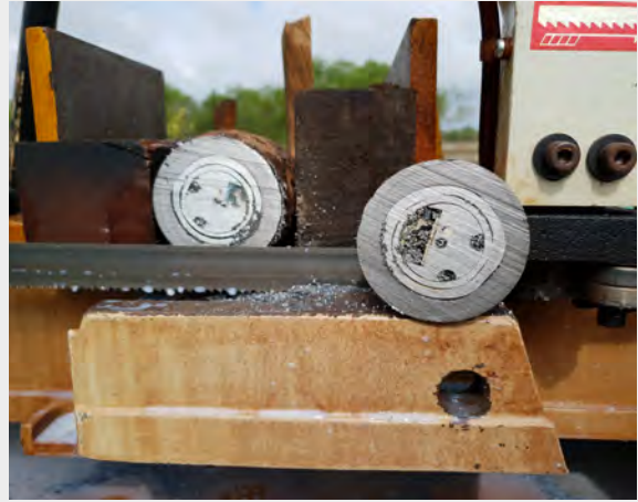
Views of the cut of the US M525 PD fuze and the booster cup section of the M374 81 mm mortar; note the damage and expansion due to corrosion of the aluminum of the fuze
