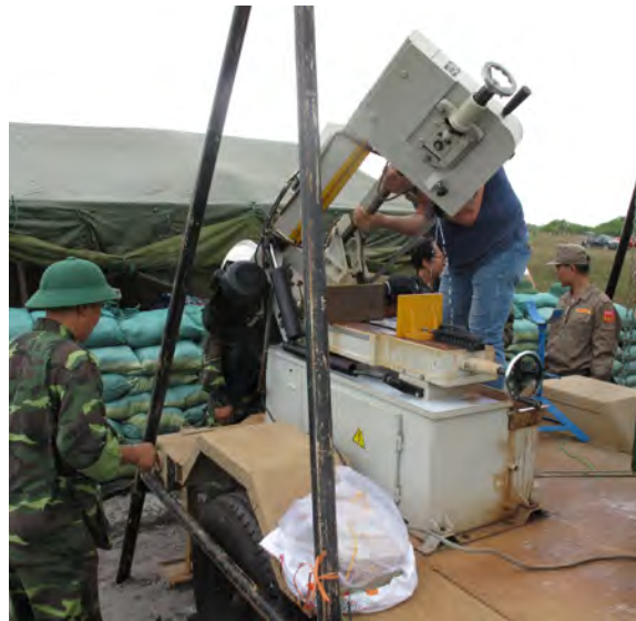
The bandsaw of the mobile cutting system
