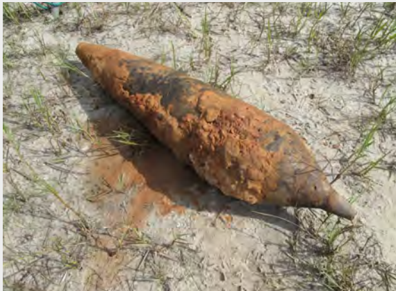
Despite the presence of caked-on mud, the body of the mortar bomb was in relatively good condition. No markings were visible
