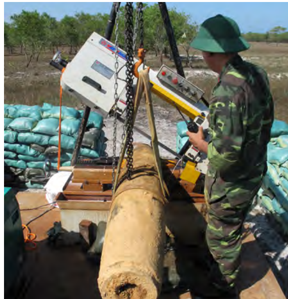
A Vietnamese soldier from BOMICEN sets up a cut on a US Mk 82 aircraft bomb
