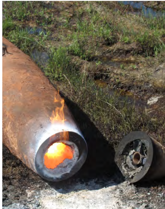
The burned-out carcass of the Mk 84 bomb as it cooled. Note that the fuze in the nose section (to the right) has been deliberately initiated using the heat of the burn, in order to render it safe
