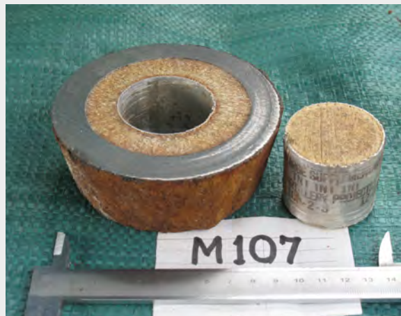
The pressed TNT boosters also remain in good condition
