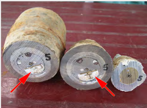
An M524 fuze, cut through the delay rotor and detonator. While many internal fuze structures remain intact, vulnerable components degrade to form expanded oxidation products (arrows); these often fill voids and seize mechanisms
