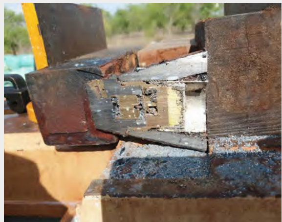
Drone view of the cutting of the M107 155 mm projectile; image on the right shows the result of the cut of the M48 series PD fuze that was on the fired M107 155 mm projectile
