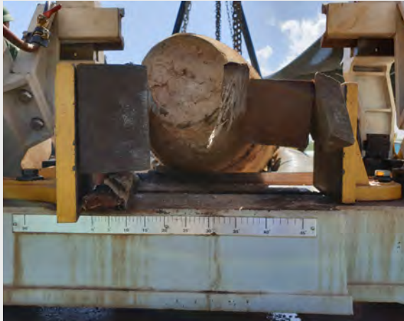
Wooden blocks were used to help hold the nose in place with the cutter clamps, as well as changing the angle of the clamps to help hold the nose steady; image on the right shows the body being slowly removed from the cutter after the successful cut
