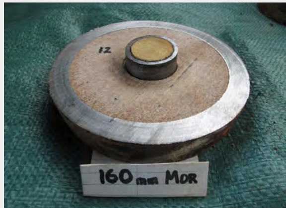
The booster cup, which is also made from steel, showed remarkably little corrosion
