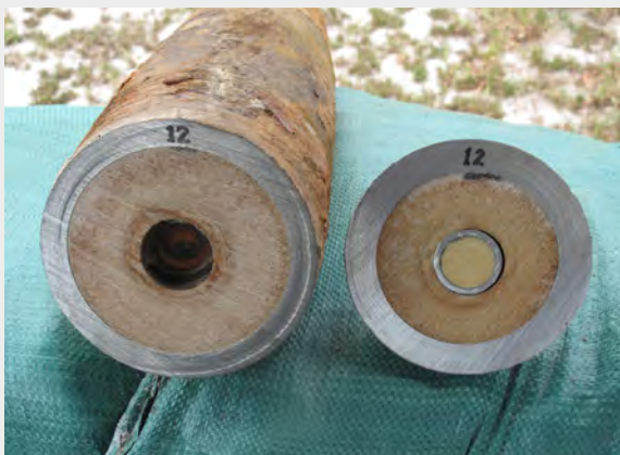
The main charge (cast TNT) and the booster were in good condition
