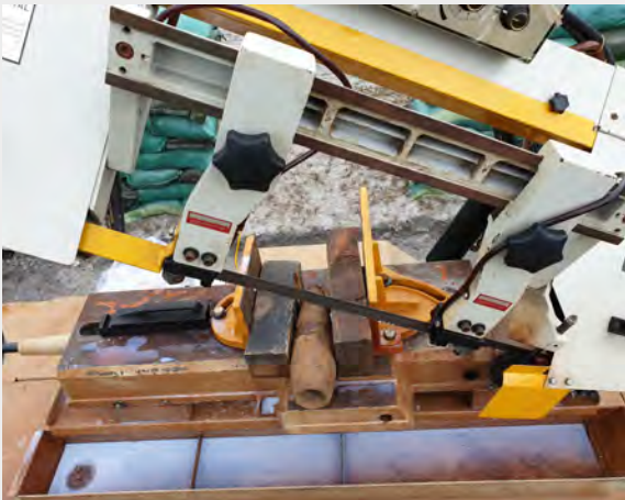
Before and after a cut of the M374 81 mm mortar
