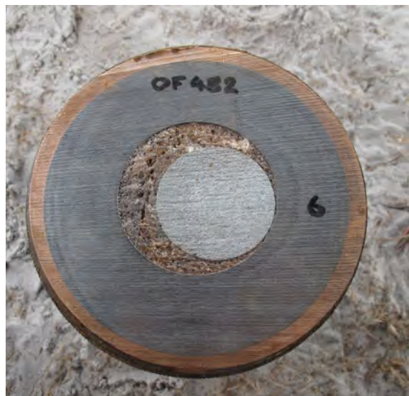
Cutting allows the visualisation of internal components, such as this incendiary pellet
