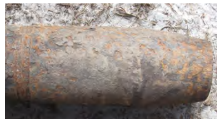
A projectile with the driving band removed
