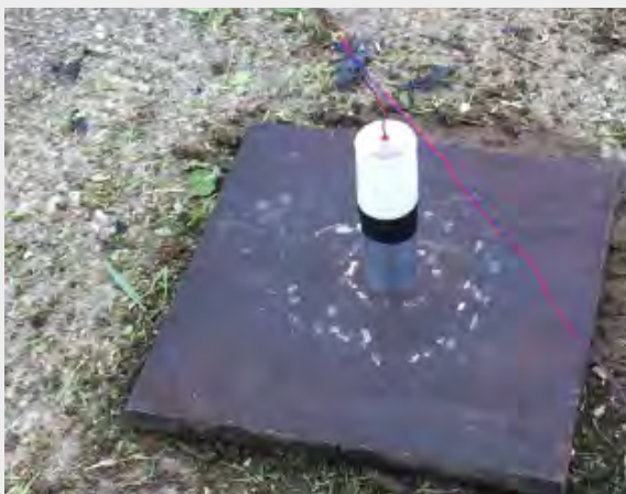
Figure 4. Sample explosion, lead cylinder compression measurement.
