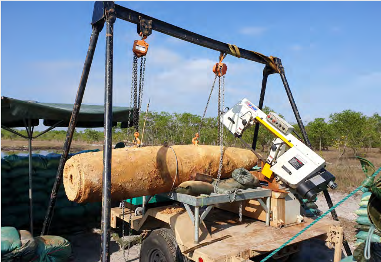
Prepping the Mk 84 2,000 lb bomb for cutting; note the use of 2 x 1-ton chain hoists and a table with sandbags to hold the bomb in place. It was important to make the bomb stable even when finished with the cut, so that it would not damage the cutter by moving or pinching the blade.
