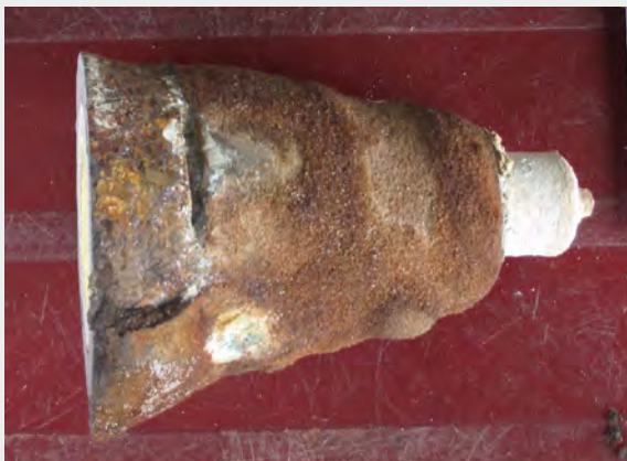
This M526 fuze was remarkably undamaged, with just the ballistic cap missing to expose the firing pin. Further investigation would be needed to establish the viability of the fuze
