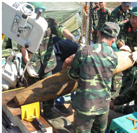
Soldiers from BOMICEN gradually assumed greater responsibility, and conducted the cutting of the second Mk82 bomb virtually unaided
