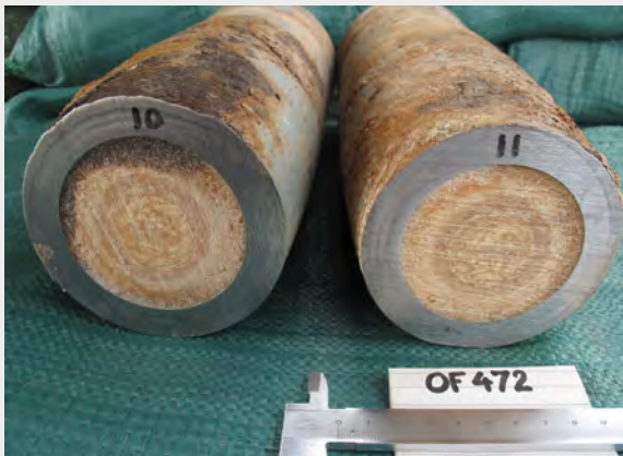
Rusting has made little impression on the thick steel casing, although water may still enter via the fuze well
