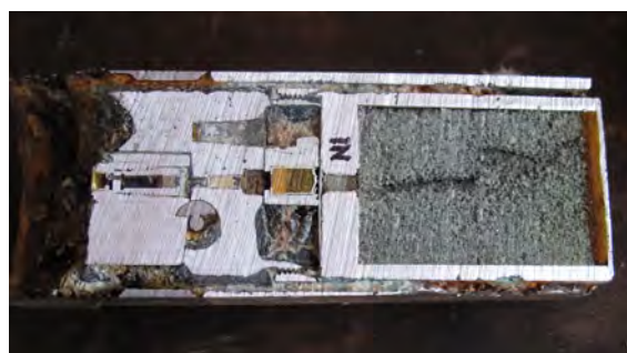
A sectioned fuze mechanism from an Mk 82 bomb, blocked by the build-up of oxidised aluminium
