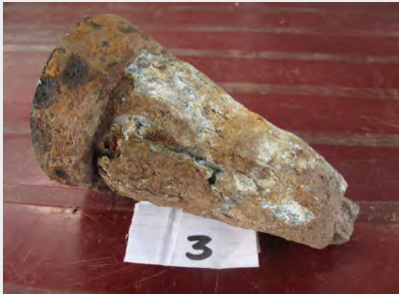
M524 fuze. The external portion of the fuze is normally damaged on impact, and may be missing altogether. The alloy fuze body is vulnerable to degradation
