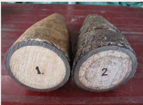
Sample #1 shows virtually no degradation while the internal corrosion, caused by the ingress of water into sample #2, has cracked and discoloured the main charge
