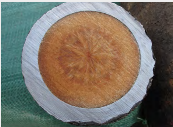
The main charge of the projectile shows no obvious signs of degradation. The pattern seen in the explosive is produced as the molten filling cools
