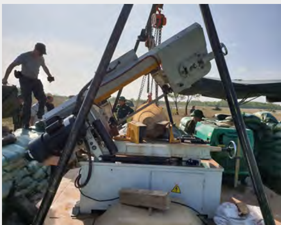
Front view of the cutting of the Mk 84. It was important to keep the bomb straight and as even as possible so as not to damage the cutter or the blade; image on the right shows the cutting blade with the metal lubricant evenly distributed throughout the length of the blade while cutting; the cut took 50 minutes due to the 22 mm thickness, and the slow drop and blade speed settings that we used for the cut.
