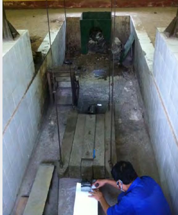
Figure 5. Determination of the ability to explosion energy with the articulation pendulum.
