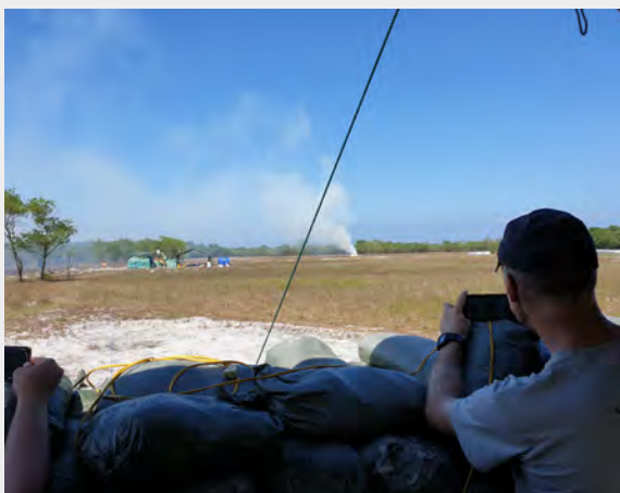
After the cut, the Mk 84 2,000 lb bomb was burned out along with the nose section containing the fuze; the Mk 84 bomb contains 429 kg of either Tritonal or H6 filler (this particular bomb contained Tritonal) and it took 40 minutes to burn out; the nose fuze detonated as required during the burnout. The image on the right shows the intense heat on the inside of the bomb casing even after the burn; note the bomb section that was cut off, containing the M904 nose fuze which was destroyed during the burnout process, to the right of the body.
