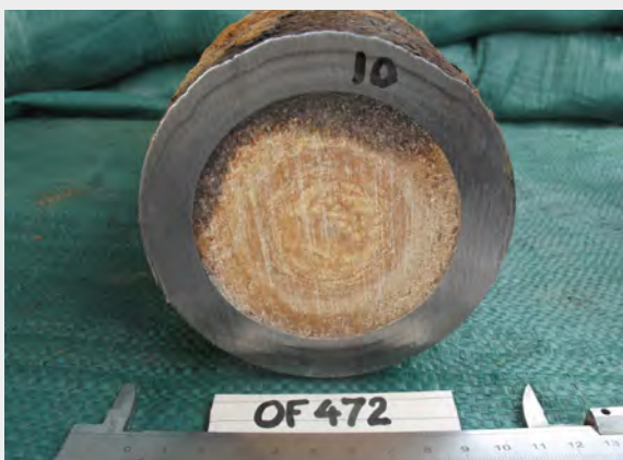
The main charge of cast TNT is slightly porous, and has allowed some water ingress over a prolonged period
