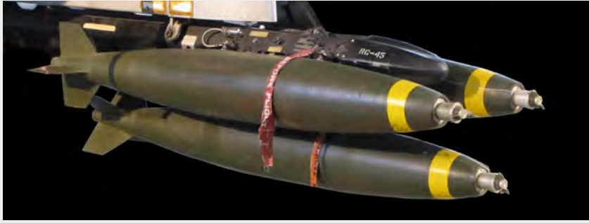
The appearance of typical nose-fuzed Mk 82 bombs before deployment
