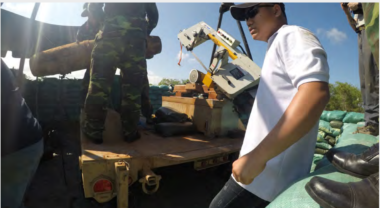
Removing the two pieces of the Mk 82 500 lb bomb after the cut
