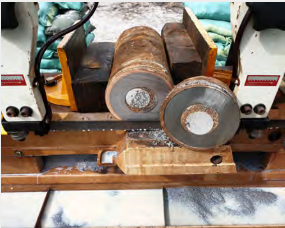
The base cut of the OF 482M 130 mm projectile showing the TCU incendiary plug embedded within the TNT filler. Also pictured is the M107 155 mm projectile with the cut at the booster cup and its HE filler
