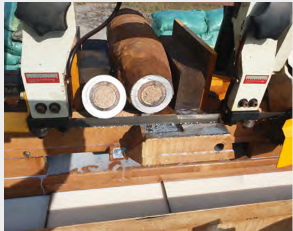
The base cut of the OF 482M 130 mm projectile showing the TCU incendiary plug embedded within the TNT filler. Also pictured is the M107 155 mm projectile with the cut at the booster cup and its HE filler
