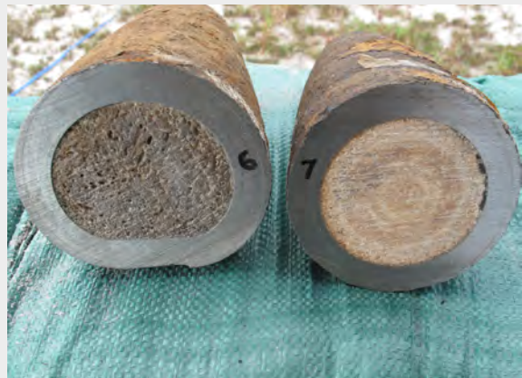
Impact has bent the casing of projectile #6, crushing the filling and allowing water to permeate throughout
