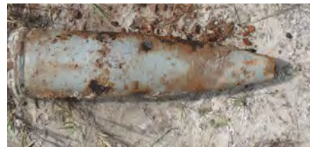
Paint and markings are among the first identification features to be lost as the casing corrodes
