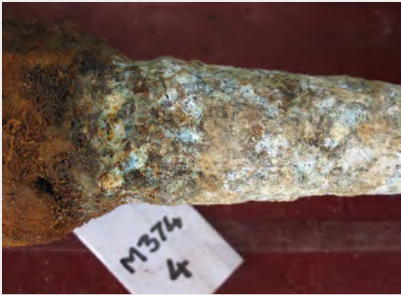
Alloys can degrade rapidly under some conditions, with the expansion of oxidised material disguising the original shape, and complete loss of material in some instances
