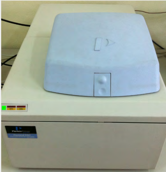
Figure 1. Differential calorimeter scanning device DSC Diamond (USA).
