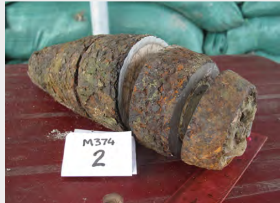
It is not unusual for the external portion of the fuze to be missing altogether. However, detonators may still remain within the section hidden by the casing
